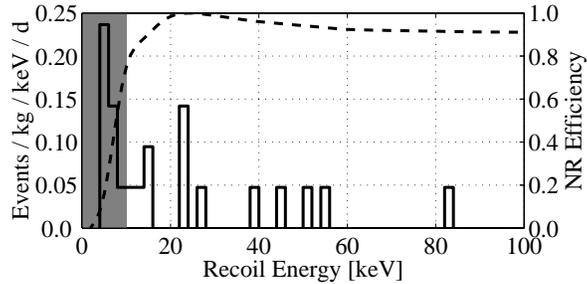
FIG. 2. Solid: histogram of nuclear recoils observed in the inner electrodes of the 3 uncontaminated Ge detectors (left-hand scale). Shaded: 10 keV analysis threshold. Dashed: peak-normalized nuclear-recoil efficiency (right-hand scale).
