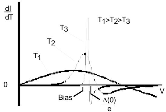
Figure 1: Current Responsivity of an SIN Junction
