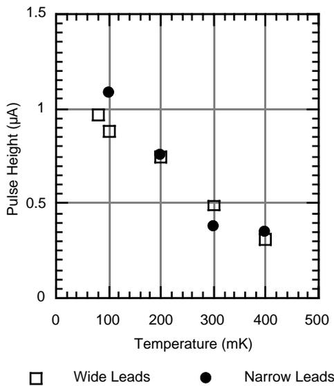
Figure 2: Pulse Height vs. Temperature
