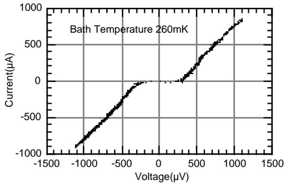
Figure 2: Typical SIN I-V Characteristic
