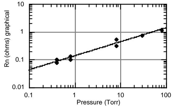
Figure 4: Rn vs. Oxidation Pressure
