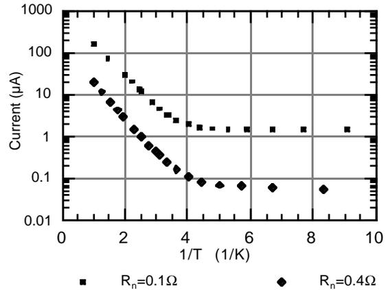
Figure 3: Current @30µV for SIN Junction Pairs
