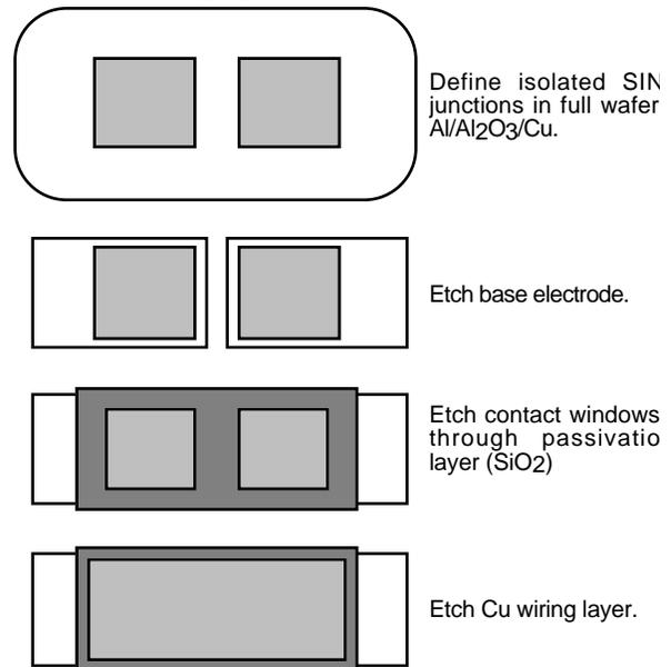
Figure 1: Etching steps for series pairs
