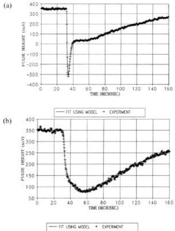
FIG. 2. (a) Characteristic pulse from particle penetrating GeAu thermistor and depositing energy directly in the thermistor itself. (b) Characteristic pulse from nonpenetrating particle.
